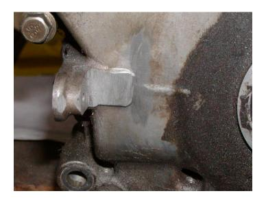
Measure over 4.140" from the center of the crankshaft and make a mark on the crank sensor mounting boss. This mark will indicate how much of the boss must be removed for proper clearance. The boss must be ground down to within .070" of the surface of the timing cover for proper clearance on the rear of the dampner. We also suggest checking the height of the factory TDC and 10\* timing marks higher up on the cover and reducing the height of these cast in marks as needed.
