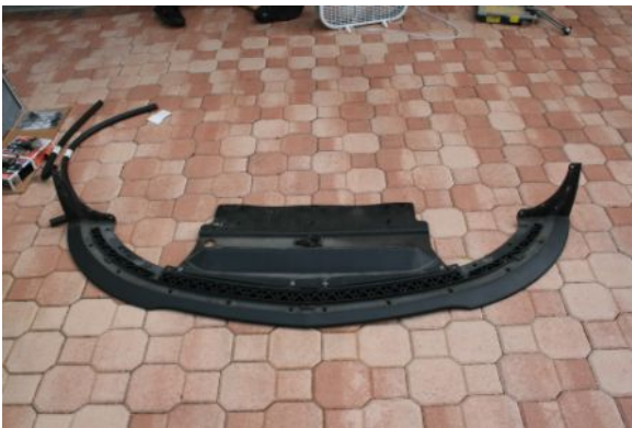
Belly pan and front splitter removed
