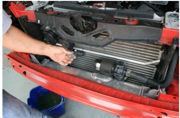
Disconnect electrical connection to water pump
