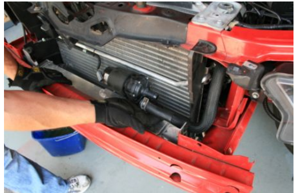
Disconnect inlet from Supercharger Reservoir to water pump
