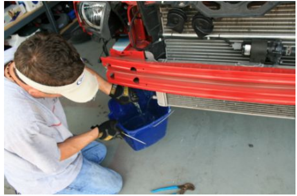
Remove clamp at bottom of heat exchanger and loosen supercharger reservoir cap and place bucket underneath to capture fluid
