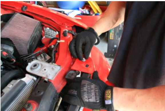
Remove upper bumper mounting screws
